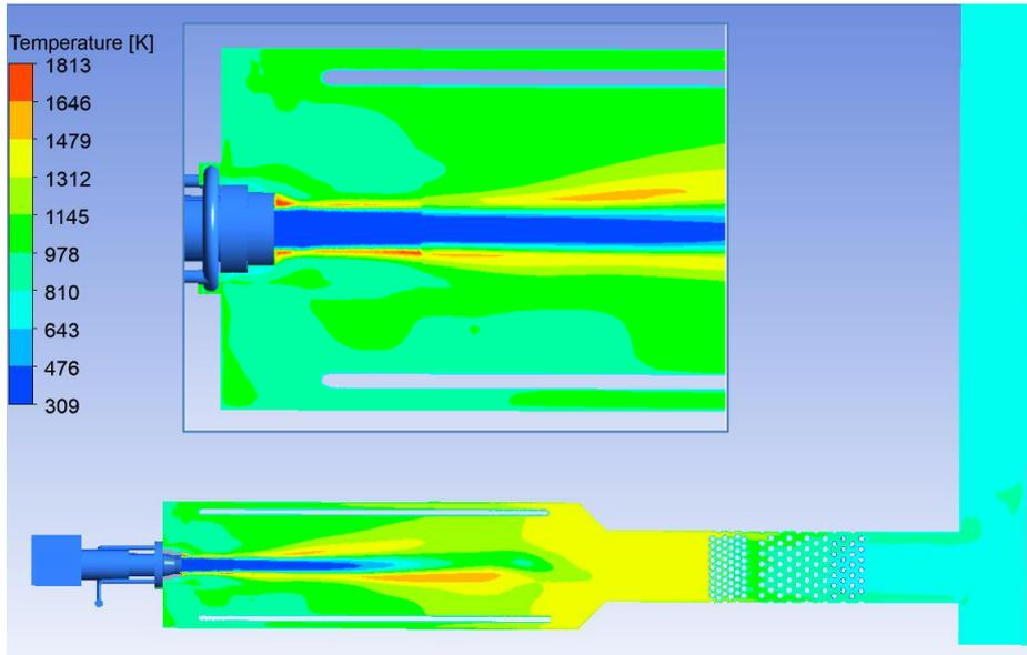
Figure 17: Temperature contours in vertical cut in the middle of OTSG
