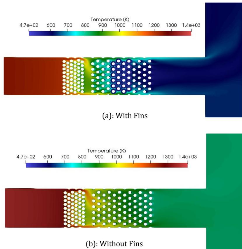
Figure 19: Temperature distribution in convection box with and without fins on the first tubes
