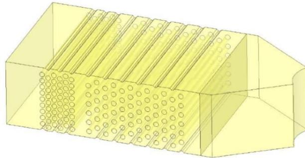
*Figure 7: Convective Section of OTSG – solid model*
