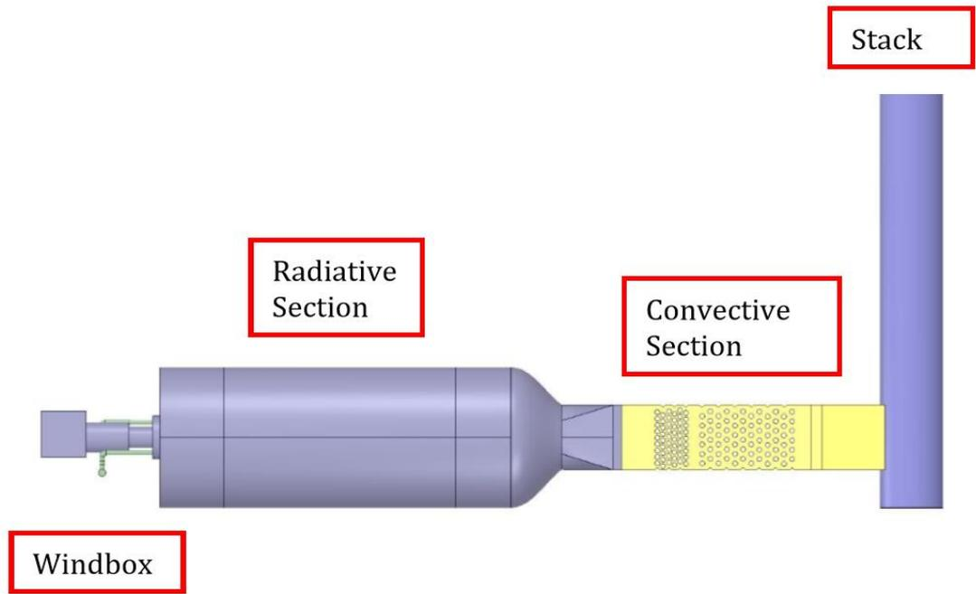
Figure 4: OTSG CAD Model for Fire Side
