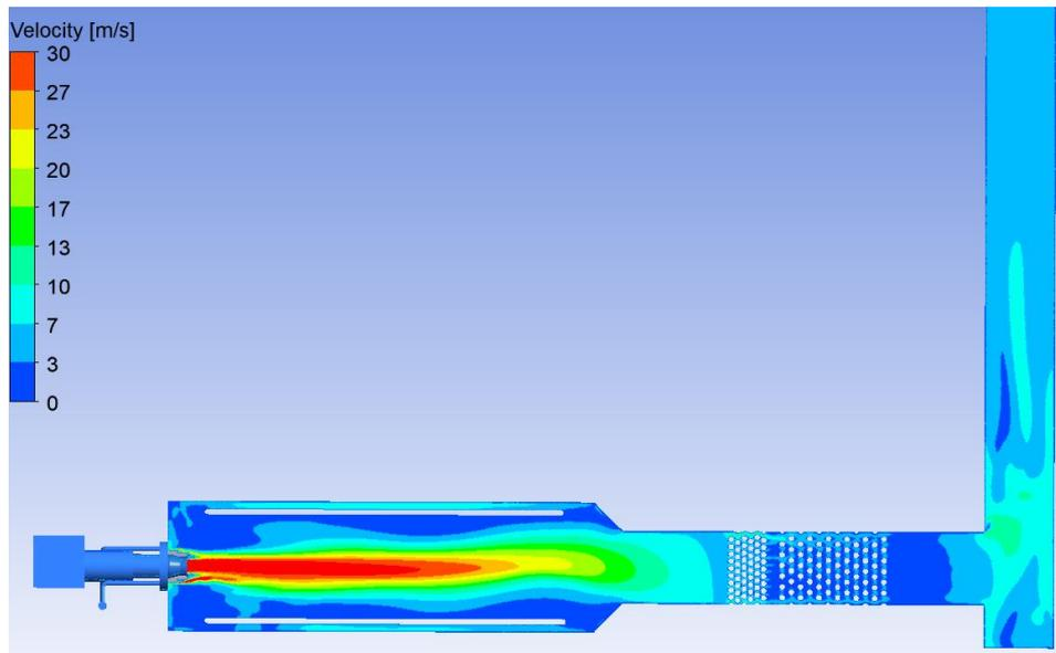
*Figure 16: Velocity contours in vertical cut in the middle of OTSG*
