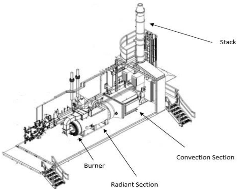
*Figure 1: Schematic of the proposed OTSG showing corresponding sections*
