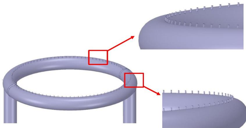
Figure 5: Burner solid model (Inset shows the close-up of the burner tips: (top=type 1, bottom=type 2))
