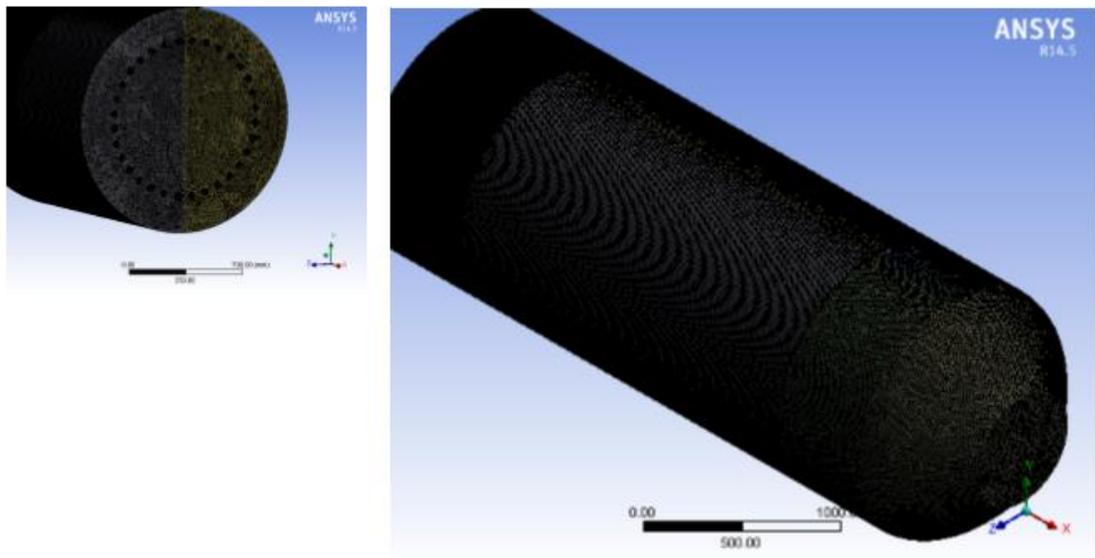
Figure 11: Fire Side Mesh for Radiant Section
