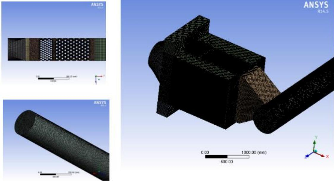
Figure 10: Fire Side Mesh Grid for Convection-Stack Section
