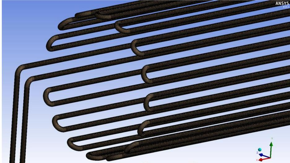
*Figure 14: Mesh Grid for Radiant Tubes*
