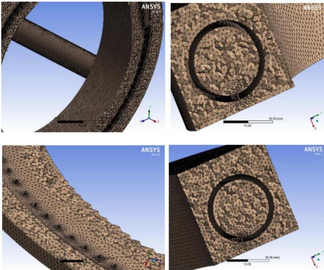
*Figure 9: Mesh-Close up of the interior mesh of fuel gas ring showing the burner tips*
