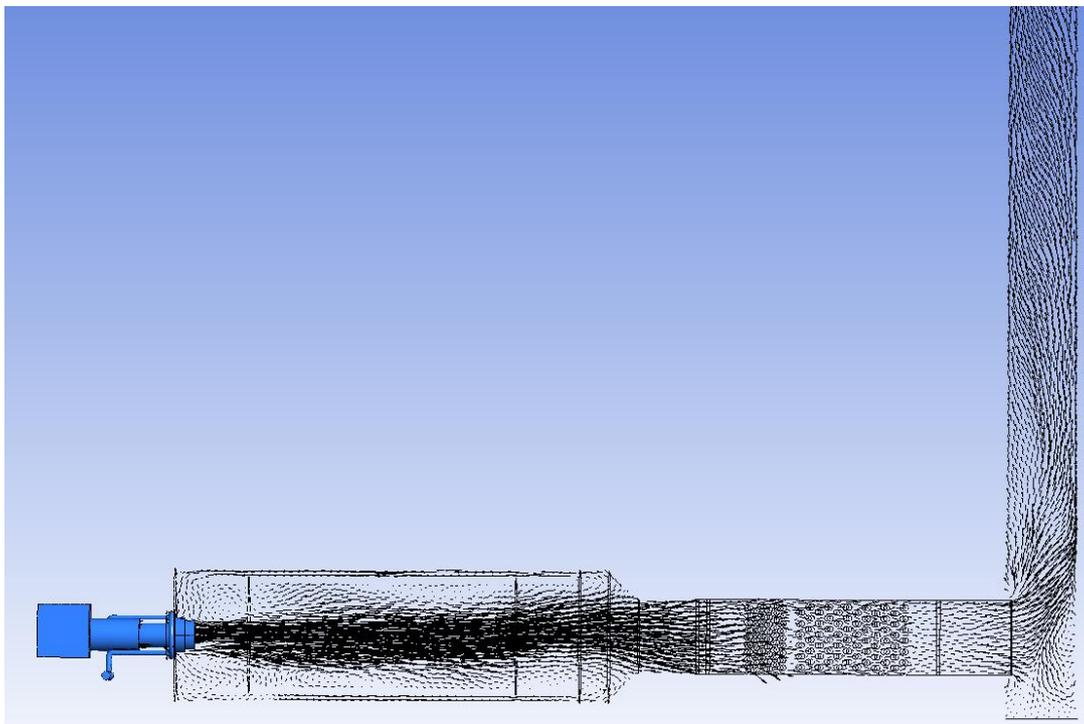
Figure 18: Vector vectors in vertical cut in the middle of OTSG
