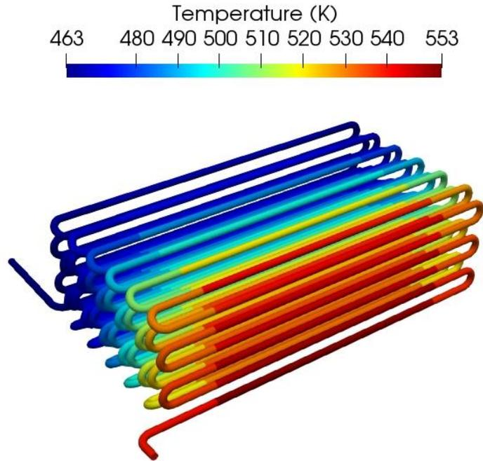
Figure 21: Temperature contours within first tubes in convention box— whole pipes
