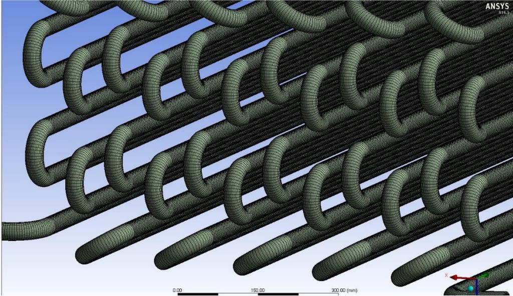
*Figure 12: Mesh Grid for First Convection Tubes (Second Tubes)*
